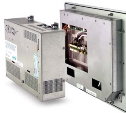
Detachable Display for Easy Replacement
